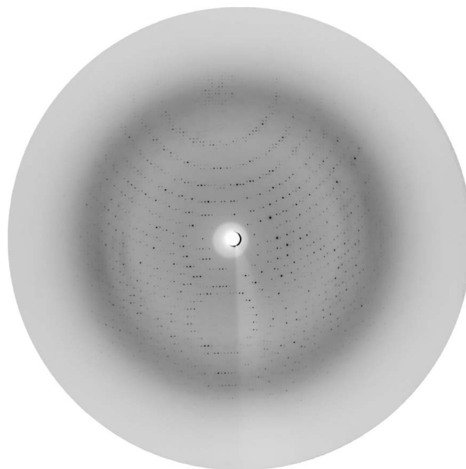
Figure 4 A typical diffraction image obtained from the HbpS native crystals. This image was collected on beamline BW7A, EMBL-Hamburg, under cryoconditions (100 K) from a single crystal mounted directly from the crystallization conditions described. Exposure times were approximately 300 s, dependent upon the storage-ring intensity, for an oscillation range of 0.2°. The incident wavelength was 0.98 Å and the resolution at the edge of the detector was 2.2 Å. Further details of the data-collection parameters are given in Table 1.
